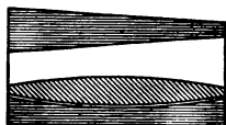
FIG. 41. — The objective spectroscope consisting of an object glass, with a refracting prism in front of it, by which the light of a star may be dispersed before it enters the telescope.
